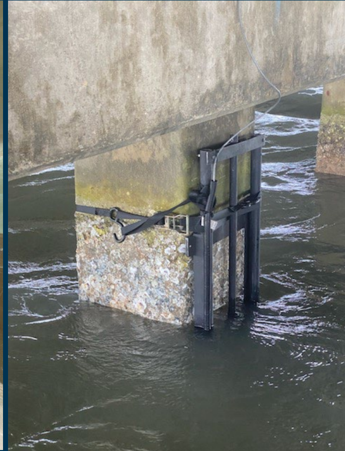
(Left): system configuration process via Sontek's SL Program (Right): shows the installed canal mount with the submerged ADCP; photos taken by advisor Dr. Jude A. Benavides and student volunteer Bridgett Collis (2022).
