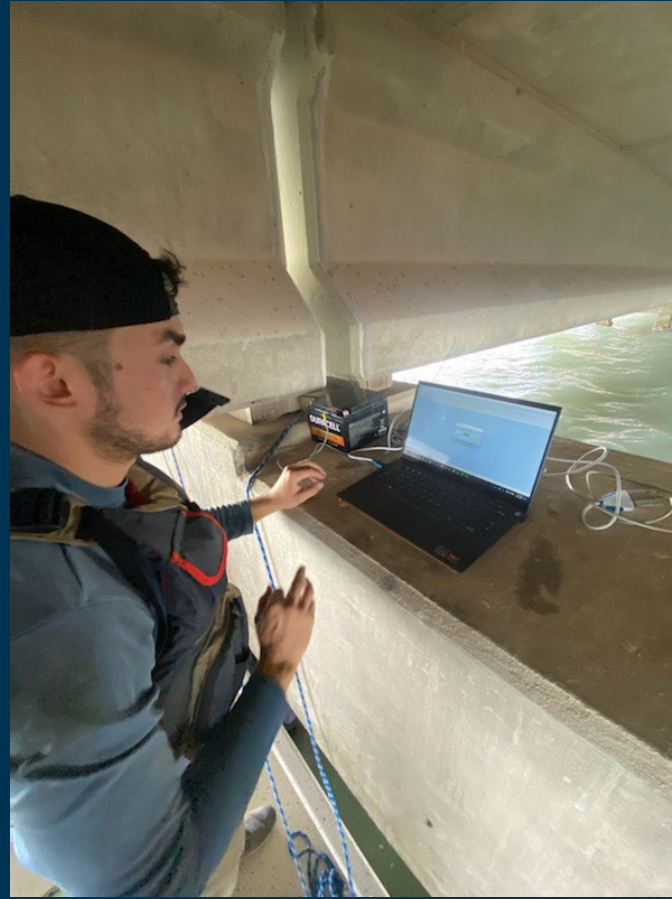
(Left): system configuration process via Sontek's SL Program (Right): shows the installed canal mount with the submerged ADCP; photos taken by advisor Dr. Jude A. Benavides and student volunteer Bridgett Collis (2022).
